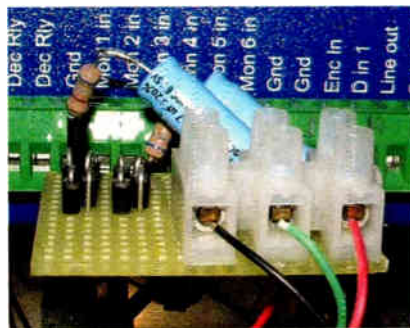
Fig. 4: This ‘Euro’ connector has a screw that pushes down on a brass tab within the port. The tab makes contact with the wire.
