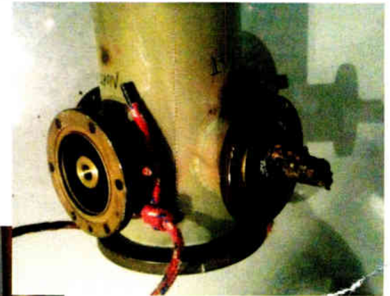
Photos above and below reveal the damage to the power divider.
