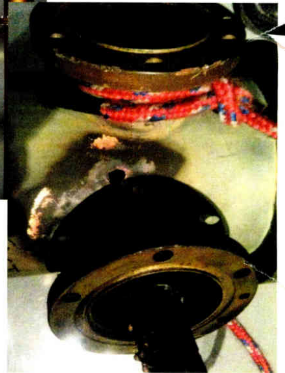
Photos above and below reveal the damage to the power divider.
