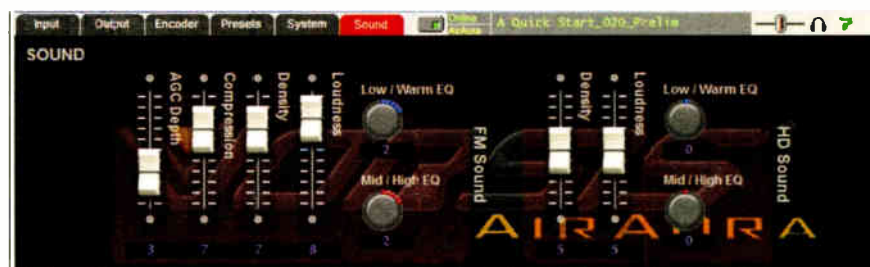
The Lite GUI interface for routine adjustments. The ‘Sound’ screen is shown.
