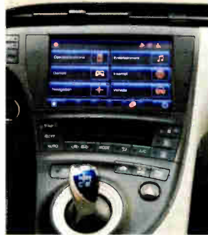
This concept car from Alcatel Lucent connects to the world through an embedded 4G LTE wireless link. It has touchscreens with buttons for functions like e-mail and Internet media – but no AM/FM.
