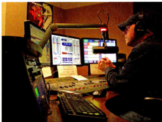
KUNV Host Greg Magnusson sits at the HD1 air studio's Axia control surface. ENCO Systems automation can be seen in the background. The mic is a Shure SM7B, its arm is a m!ka with a tally light.
