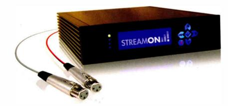
hardware (appliance) required an Internet connection with its own static IP address, connection to our automation system Scott Studio SS32 for playlist data and an audio connection (XLR balanced). I installed the audio after our Omnia 6 audio processor to make sure that the audio into the appliance was the same as what we put to air.
