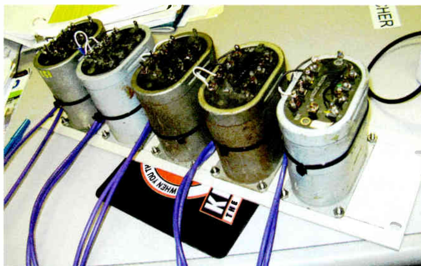
Fig. 1: Kill the hum using old WE111C repeat coils.
