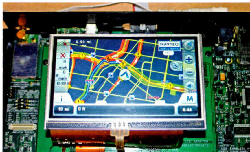
The HD Radio power boost is intended, among other things, to help support next-gen data services. This is an ST Microelectronics-based HD Radio receiver development board showing Navteq traffic information displayed at CES.
