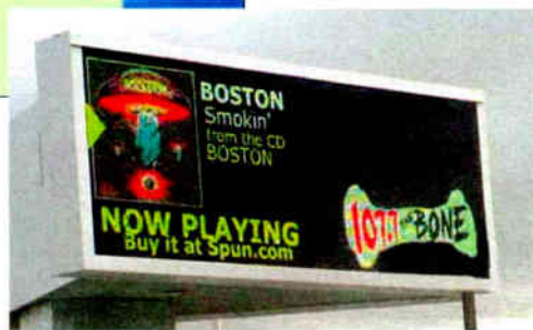
Right: Interactive billboards may be controlled by the group 5A subset of RDS, or if they are connected to the Internet, via XML files.
