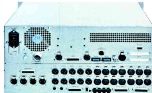
Backplane of the Rackmounted Mainframe Input/Output and Processor Box
