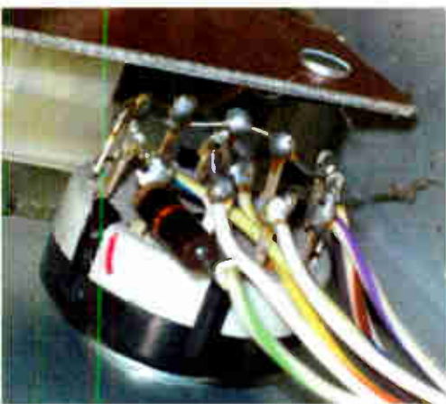
Fig. 4: Adding a resistor, foreground, to the meter switch ends pegged meter indications.
