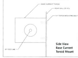
The current transformer obviously wouldn't stay in place by itself, 18 inches up on the back wall, in order to let me thread the mounting bolts back into its base. The bolts mount through the rear side of the metal ATU box and into the current transformer base. Unfortunately the ATU was too large for me to reach around the back to start the bolts while holding the transformer in place. I was stuck.
