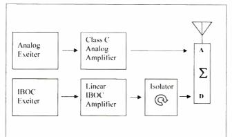
Fig. 3: Dual Input Antenna
