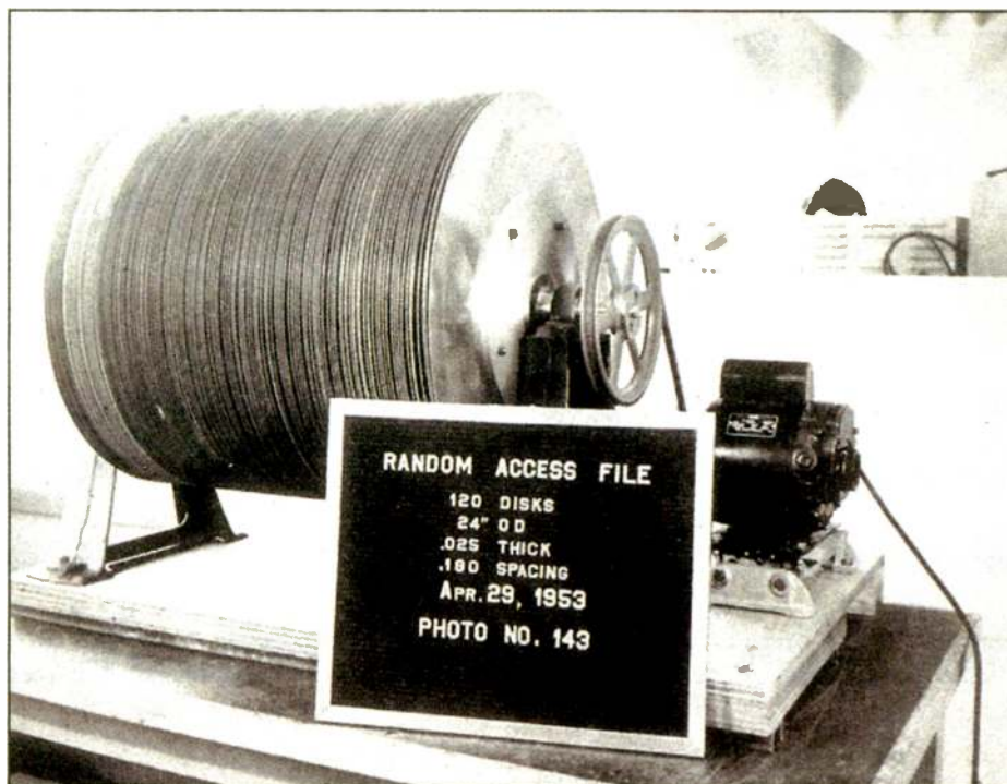
Early laboratory assembly of a disk drive that would become part of the RAMAC computing platform.
