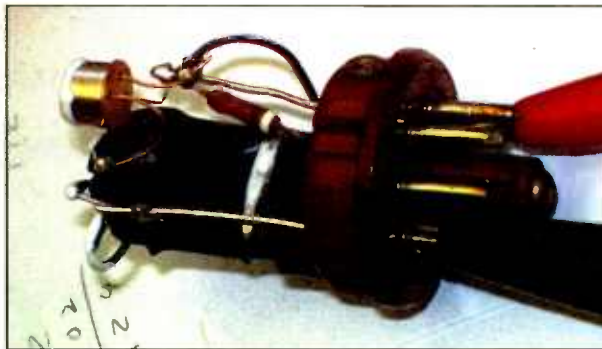
Fig. 2: The proportionate crystal heater undergoes bench test prior to final assembly.
