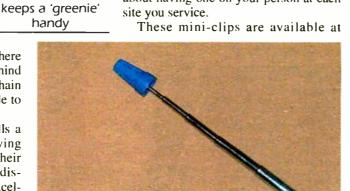
Fig. 2: This wire nut on the end of a broken antenna prevents the end from collapsing.
