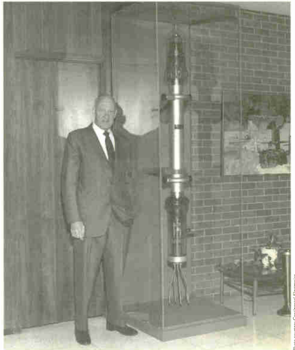
James O. Weldon is shown with one of the massive Western Electric 320A triodes used in the 500,000 kW Doherty transmitter that he constructed for Dr. J. R. Brinkley in Villa Acuña, Mexico.
