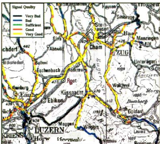
Fig. 4: Measured coverage quality of the analog FM signal of Radio Sunshine's main transmitter at 88 MHz. The different colors represent the five-grade CCIR scale for audio quality.
