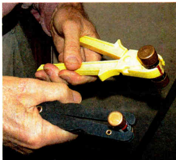
Fig. 2: An inexpensive pair of fuse pullers removes blown fuses safely.
