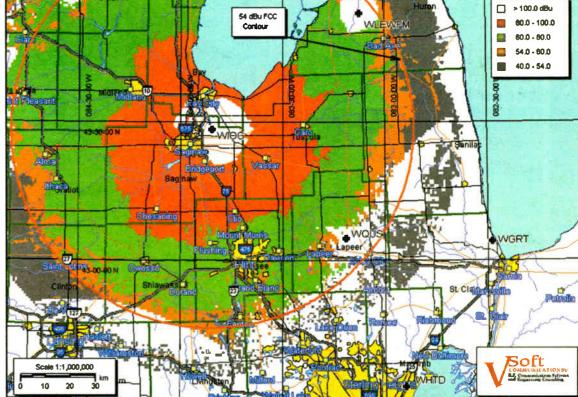
A comparison showing the "baseline" analog interference-free coverage of WIOG(FM), Bay City, Mich. while the other shows the "bites" taken out of its coverage to the southeast by all other stations' IBOC interference.
