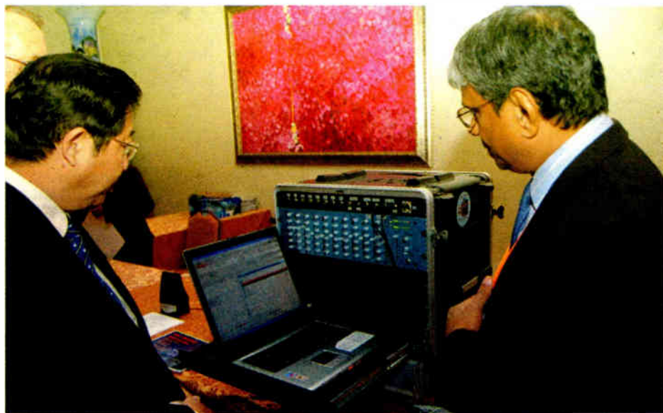
ABU showcased a 'radio station in a box' that could be transported to disaster areas to provide emergency coverage. Housed in a rugged case, it contains a solid-state transmitter, antenna, audio mixer, microphones and monitoring for a quick-start operation. Shown: Malaysian Deputy Information Minister Chia Kwang Chye, left, and ABU's Rukmin Wijemanne.
