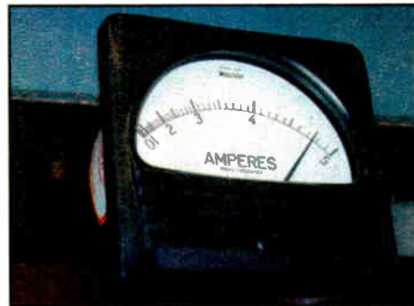
Fig. 2: Allow thermocouple meters time to warm up before reading them.
