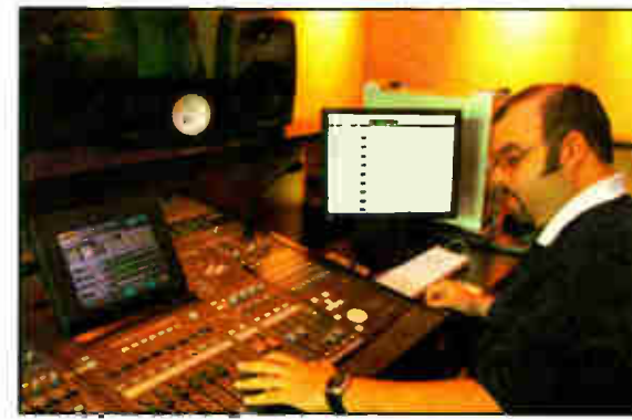
Caruso says the station uses a combination of a Yamaha PM5D digital mixing console and ProTools HD-192 system.
