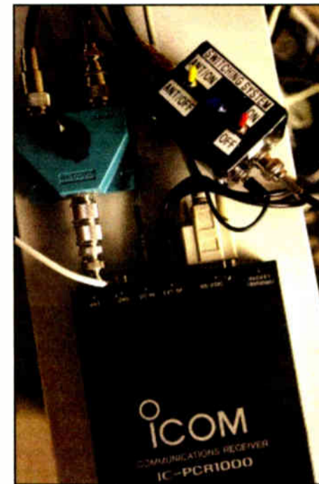
The most popular user-controlled online tuner is the ICOM PCR1000, shown here with a couple of antenna switches, one manufactured and one home-built. Don't forget to ground the system (white wire in left of photo).
