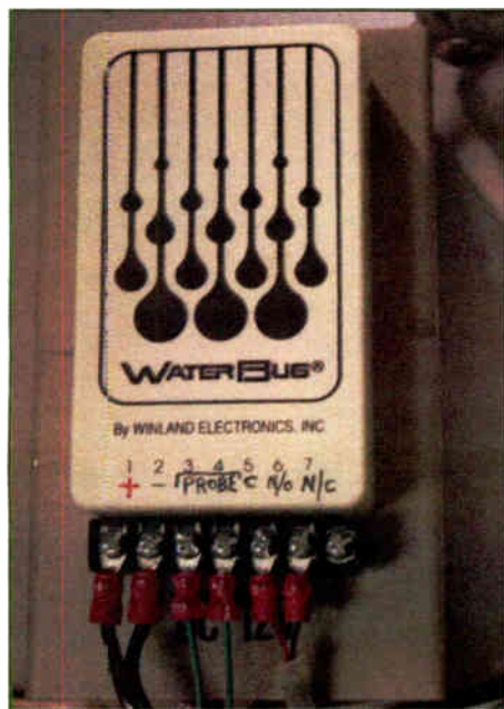
Fig. 1: The WaterBug warns of leaks by connecting to your remote control.
