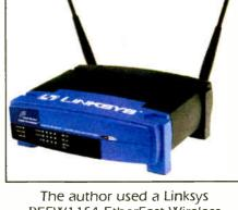
BFFW11S4 FtherFast Wireless AP + Cable/DSL Router w/4-Port Switch. It connects a wireless network to a high-speed broadband Net connection and a 10/100 Fast Ethernet backbone.
