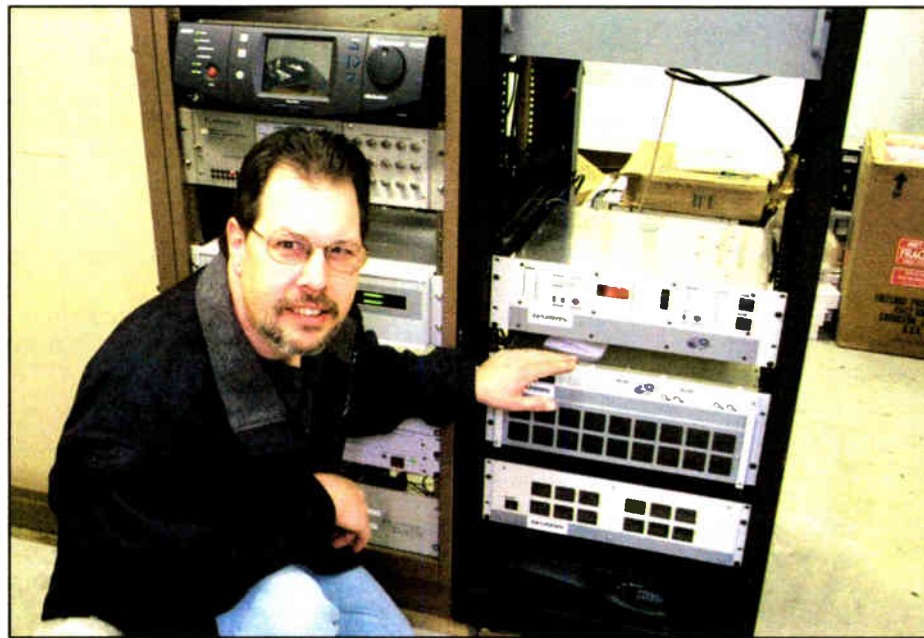
The Harris Mini-HD is a low-power HD Radio transmitter. Dave Supplee is with Cumulus Broadcasting.
