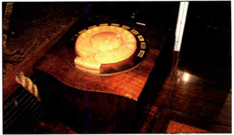
When dialed to finger-stop and released, this 6 x 8 x 4-inch remote control causes the 39-116 receiver to retune itself to the selected station within 15 seconds.
