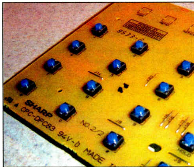
Fig. 2: A busted fax machine circuit board provides lots of micro snap-switches.
