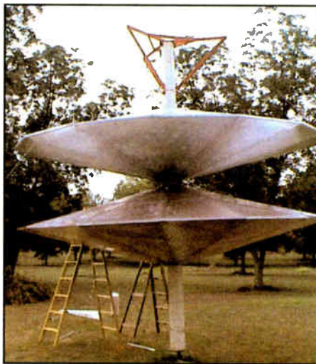
The completed disc-cone. The developer is assembling a ground-plane version, a single cone over a ground plane.
