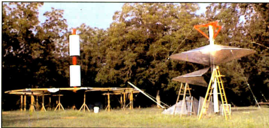
A broad view of a prototype disc-cone antenna partially finished and a dipole version over a ground plane. The final AM version would be about 8 feet tall.
