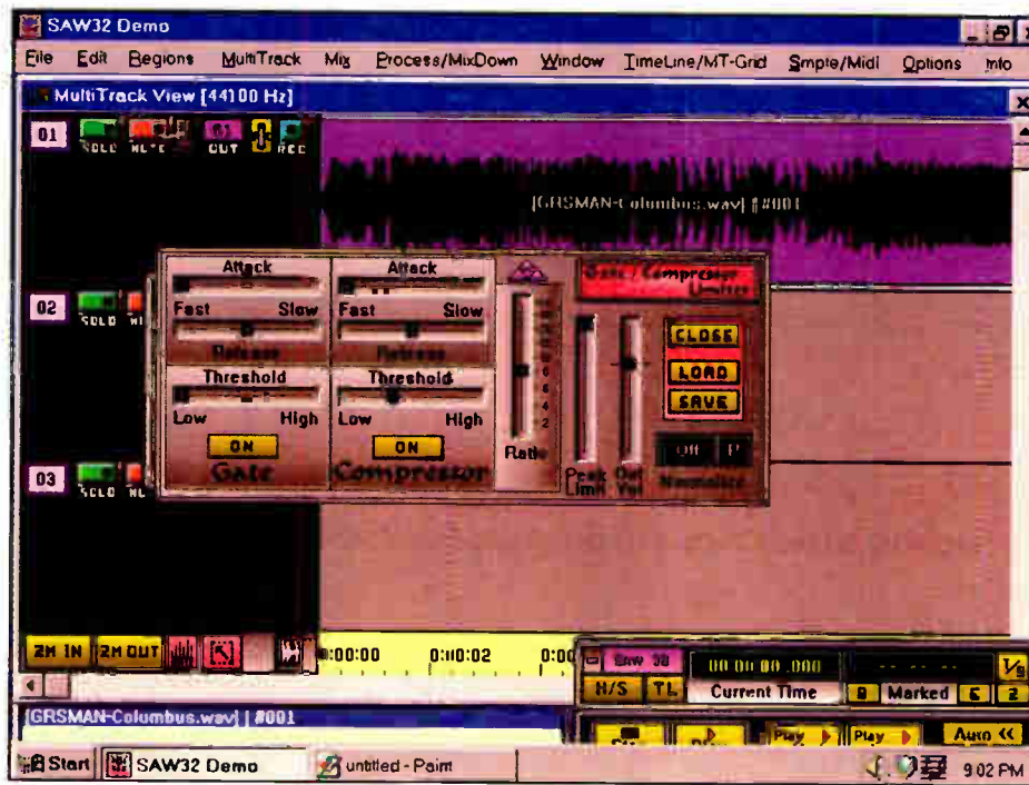
DAW programs such as the IOS SAWPlus include both compression and EQ. Voice processing can take place following the actual recording.
