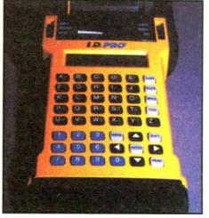
Figure 1: Brady's new ID Pro prints professional cable ID labels that are self-adhesive.
