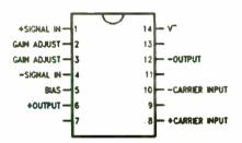
Pinout for the National Semiconductor 1496 Balanced Modulator Chip
