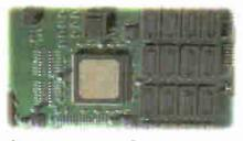
Integrity uses an array of state-of-the-art floating-point digital signal processors to perform its mixing, routing and other functions.
