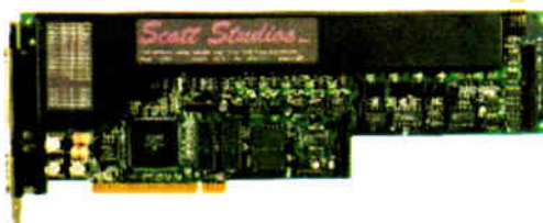
Scott Studios exclusive new 32-bit PCI audio card plays up to four CD quality uncompressed stereo channels while recording!
