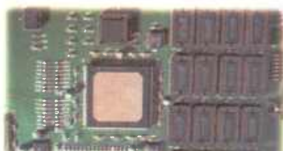
Integrity uses an array of state-of-the-art floating-point digital signal processors to perform its mixing, routing and other functions.
