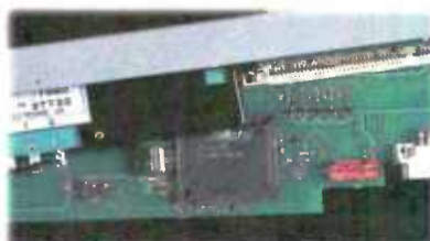
Our proprietary gate array logic generates both module control and remote control of connected equipment.
