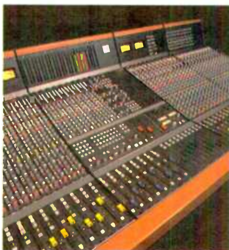
Calrec S2 60 Channel Surround Sound Console supplied for Game Greek USA mobile
