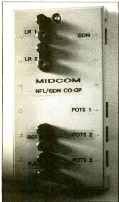
ISDN Network Termination Panel
