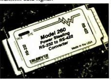
With only TD, RD and ground, the Model 260 provides operation on the RS-422 side over 8,000 feet of twisted pair into a load of 120 ohms.
