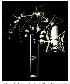
a threaded mount. A small, battery-powered remote controller links the Positioner via a conventional XLR cable. Using the controller, any microphone can be rotated through 350 degrees and tilted 180 degrees, providing full control of the capsule's orientation.
