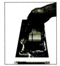
Vertically slotted plug-in cards permit easy access and service.
