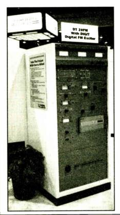
LAS VEGAS A new Harris 20 kW FM transmitter equipped with Digit™, a digital FM exciter, was showcased at the Harris Allied booth.
