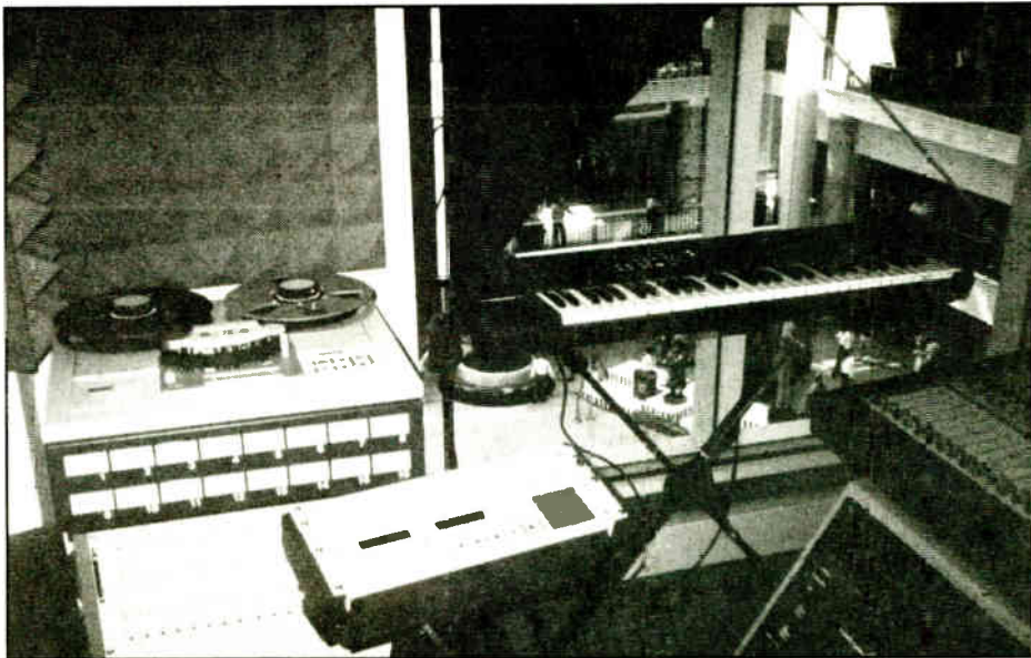
The high-tech WMMS "Zoodio" features a Tascam 16-track reel-to-reel, Mirage sampling keyboard, and a rack of effects.
