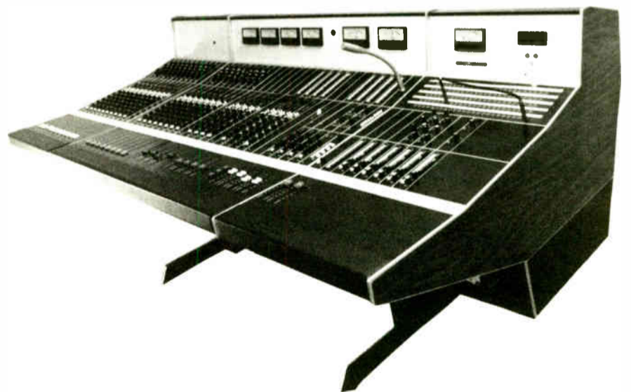
WARD-BECK Modified Type L3242A TV Audio Console
