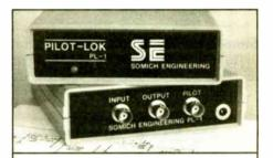
The PL-1 is a baseband filter that protects the 19 kHz pilot during moderate to heavy composite clipping.
