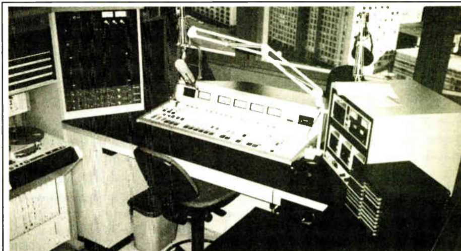
Production A uses an Audiotronics 218 (center). Turntables are hidden under lids to operator's right.
