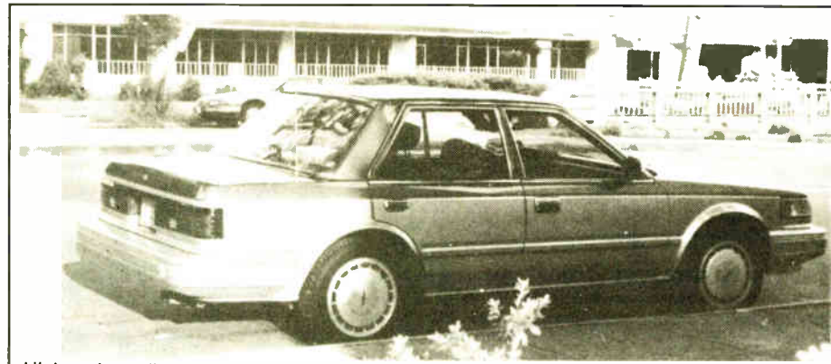
High end cars like this Nissan Maxima have diversity reception. Rear antenna and hidden window antenna allow a choice of signals.
