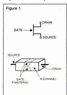
than bi-polar transistors. FETs are constructed with a drain, source and gate as illustrated in Figure 1. The devices can be made to be either P- channel or Nchannel.
