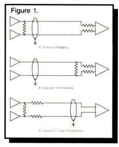
resistance and a low resistance are in parallel, the result is a value very close to the lowest resistance.
