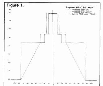
In the case of the average specification, the reference level would again be symmetrical from the carrier to  $\pm 10$  kHz, dropping to -35 dB in the range of 10 to 20 kHz. At 25 kHz, the specification would taper to -40 dB, at a rate of 0.5 dB/kHz.
