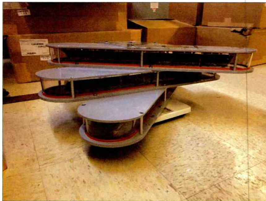
Dialight High intensity LED modules. The modules shown just came out of the box and I was trying to weigh the assembly. This is quite different from our old strobe tower lights.
