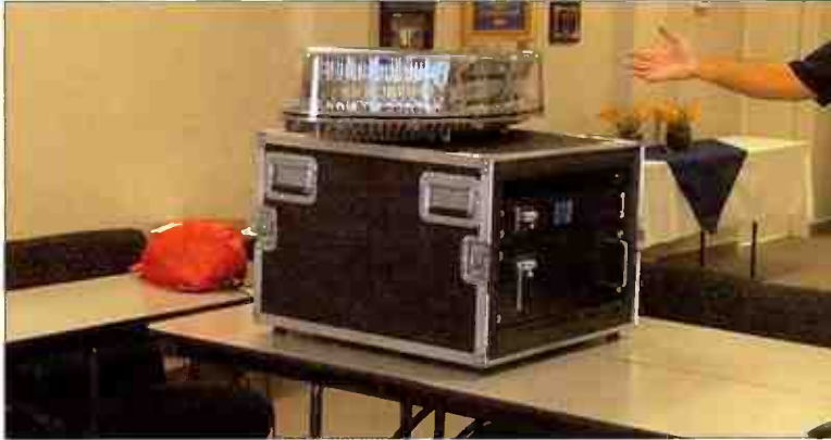
DRAKE tower light controller and LED light assembly on demo. The light assembly on top of the box covers 120 degrees on one leg of a three-legged tower. Three of them cover the whole 360 degrees around the tower.
