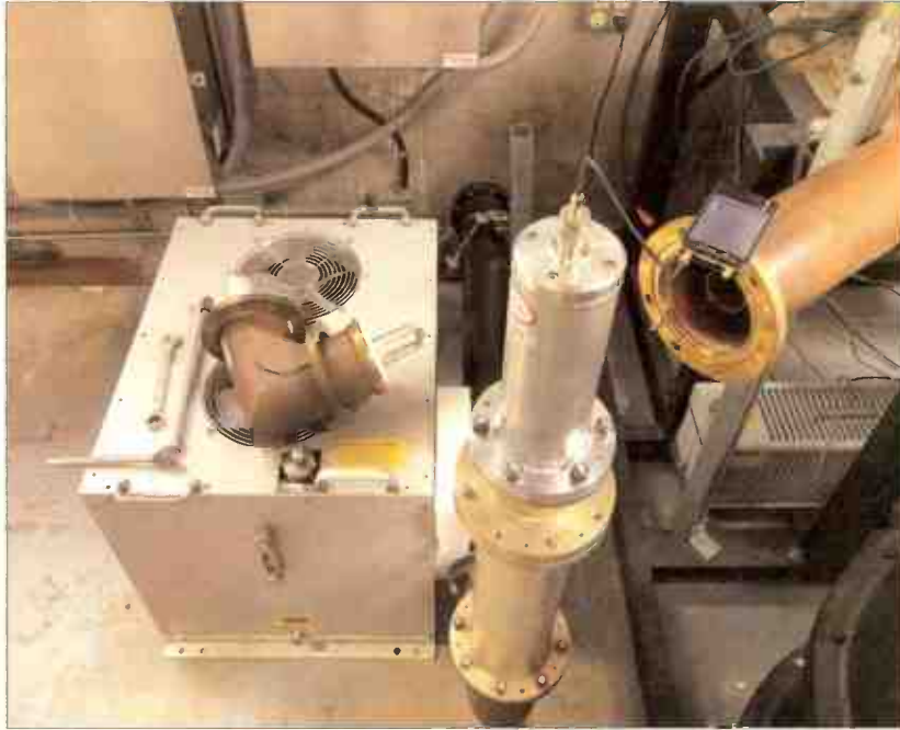
Figure 4 – Checking the impedance of the column load with my Pocket VNA.
