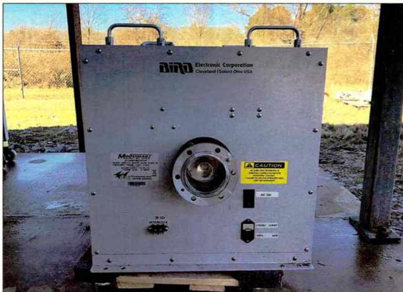
Figure 1 – Bird Moduload RF load resistor Model 8645-115. Rated 25 kW
