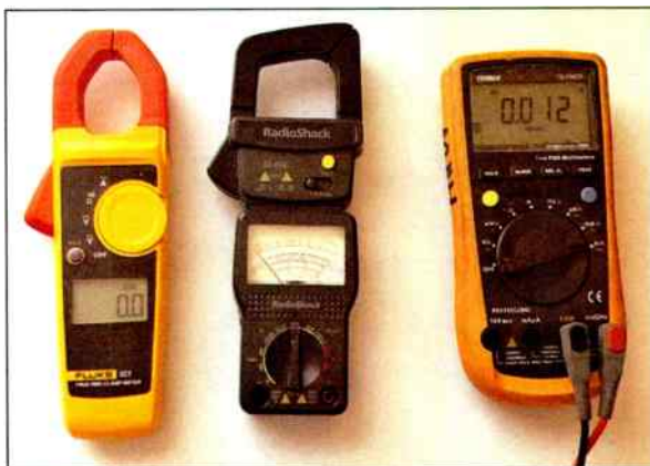
Ammeters used in measuring the ground current.
