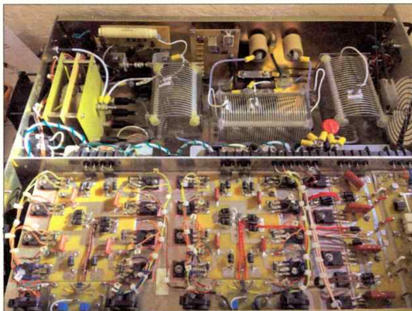
Figure 3: 1kW PWM Transmitter Amplifier box. Shown are the output network on top, two boards of RF amplifiers and the modulator board on the right side.
