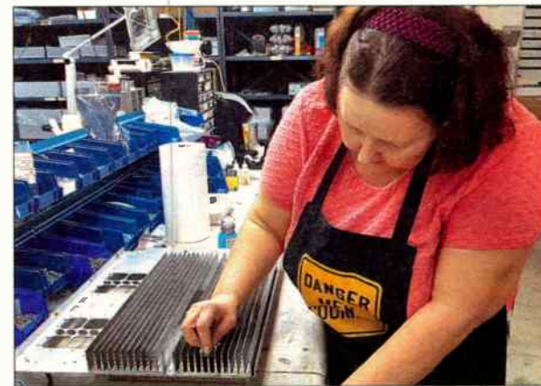
Assembling and Cleaning a 4kW Heat Sink
