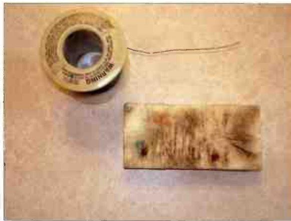
Figure 7 – Lead Free Solder & Sal Ammoniac
