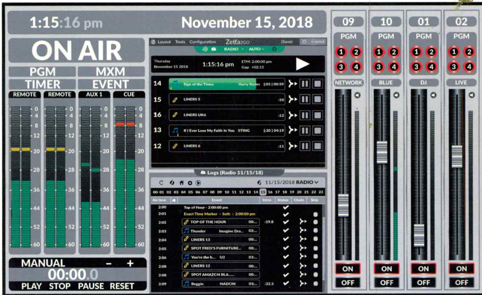
This screen provides full local or remote control over a live show, complete with specific console and automation functions. Courtesy SAVE Diffusion.
