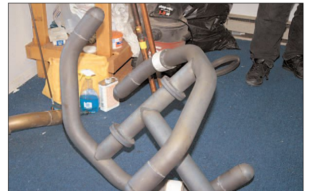
This photo shows the "Tee" section between the radiating arms of the bay. The base of the Tee is an impedance transformer.
