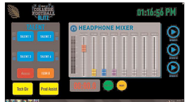
This example of the ScreenBuilder app shows how faders, meters, labels, buttons, clocks, timers and other widgets can be connected to devices and network interface points and arranged on-screen to perform functions remotely.
