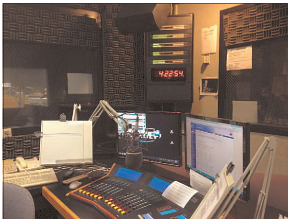
WEKU Richmond studio showing American Audio VU meter returns for each repeater (to upper left of the console).
