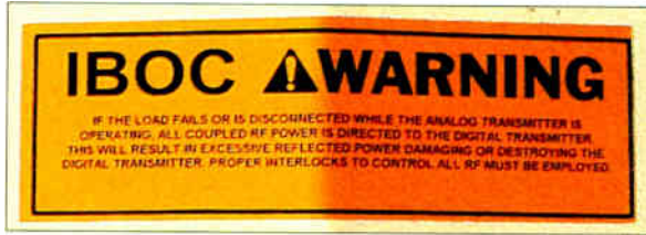
The warning label on a new Altronic dummy load.
